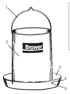
NOTE: Model HF15 is packed six (6) to a carton. If you split the carton, please be sure the correct number of parts go to the end user. Each feeder consists of 1 pan, 1 tube, 1 handle, 2 adjusting wires, and one hardware bag containing 4 speed nuts.
