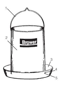
NOTE: Model HF15 is packed six (6) to a carton. If you split the carton, please be sure the correct number of parts go to the end user. Each feeder consists of 1 pan, 1 tube, 1 handle, 2 adjusting wires, and one hardware bag containing 4 speed nuts.
